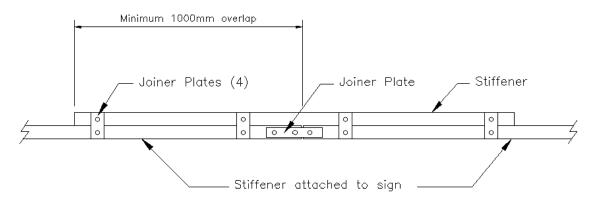
A minimum overhanging length of 1000 mm is required for the stiffeners at vertical joins
