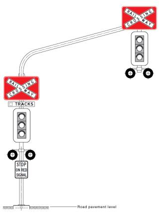
Figure 6.2 Traffic signals incorporated into an overhead flashing signal assembly
