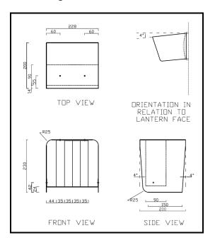
Figure 4.5 Pedestrian visor with vertical louvres for use with split approaches
