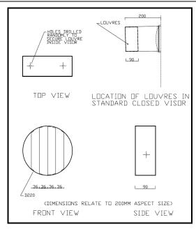
Figure 4.3 Visor with vertical louvre for obscuring signals at adjacent sites
