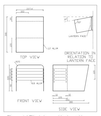
Figure 4.1 Tilted visor and horizontal louvre
