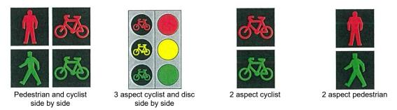
Figure 4.4 Permitted pedestrian and cyclist signal face layouts Extracted from AS 1742.14
