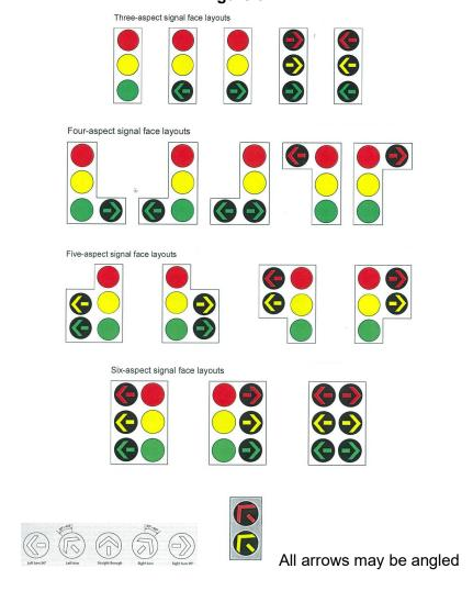
Figure 3.1 Permitted Vehicle Signal Face Layouts Extracted Austroads Guide to Traffic Management (GTM) Part 10 (2020)
