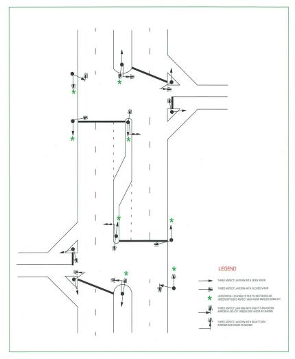
Figure 4.2 Staggered T-intersection showing the locations of tilted visors
