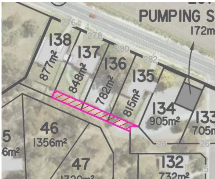
Figure 5: Proposed right of way which will service allotments fronting Woodside – Nairne Road
