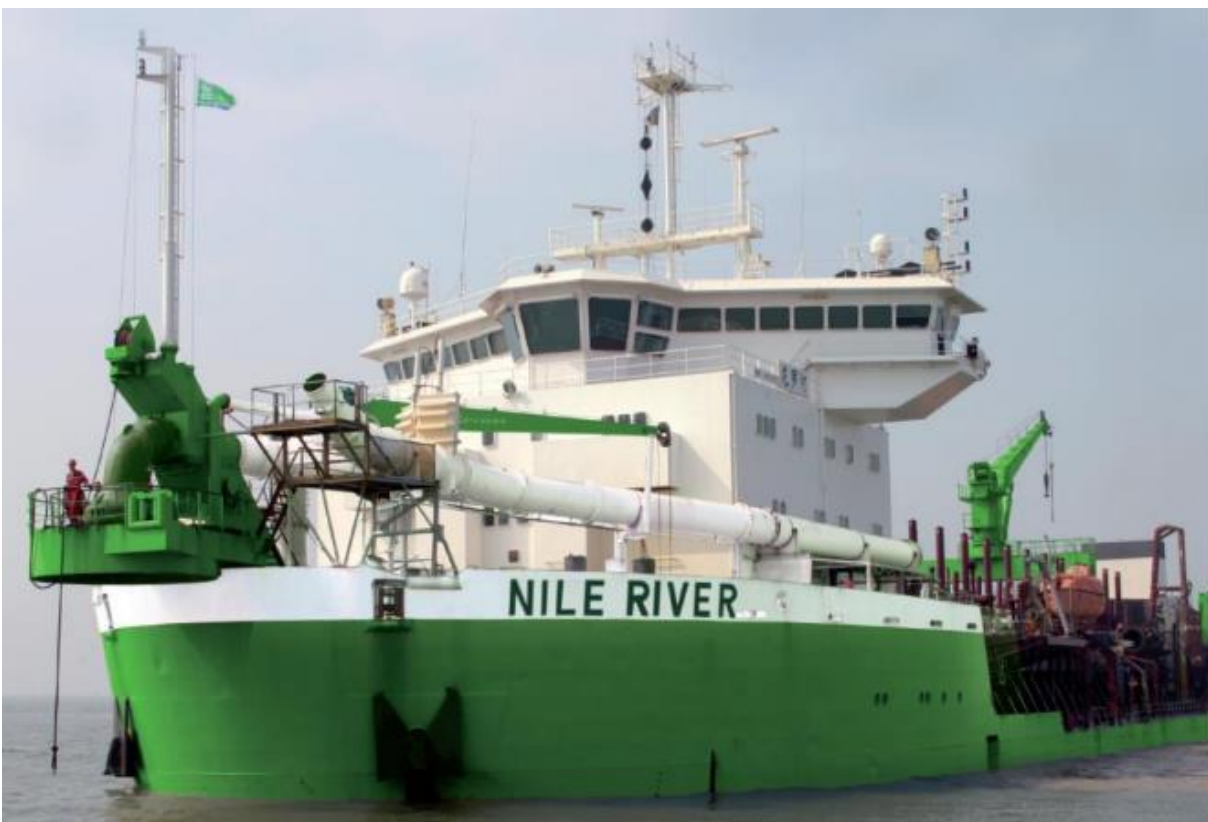
Figure 2: An example of the Trailing Suction Hopper Dredge
