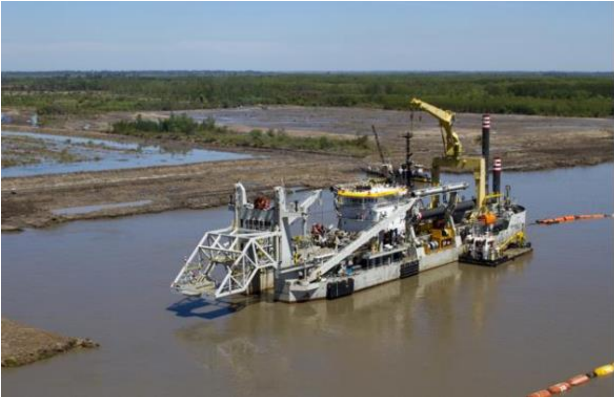
Figure 1: An example of a Cutter Suction Dredger
