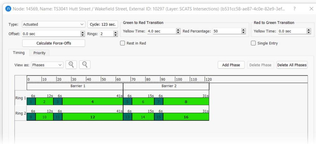
Figure 3.5-8 Example of the interphase layout for control plans in TAM
