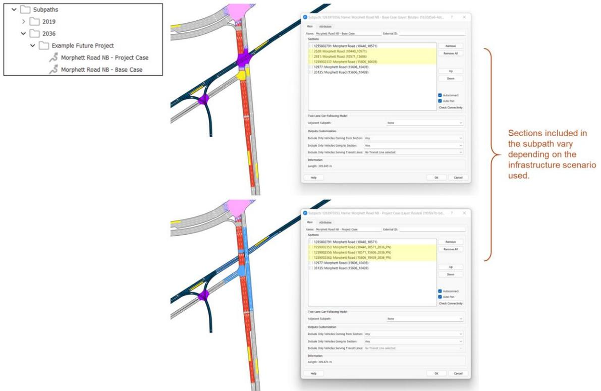
Figure 3.4-3 Example of subpaths created for base and project case geometry configurations
