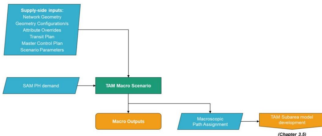
Figure 3.3-1 Overview of the inputs, processes and outputs for a TAM Macro scenario
