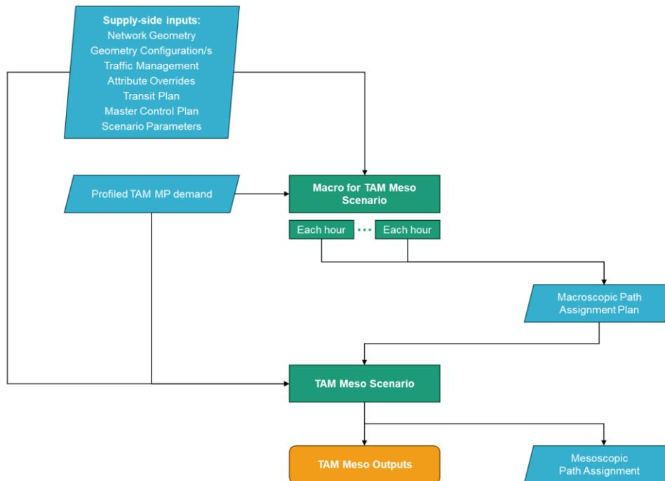
Figure 3.4-1 Overview of the inputs, processes and outputs for a TAM Meso scenario
