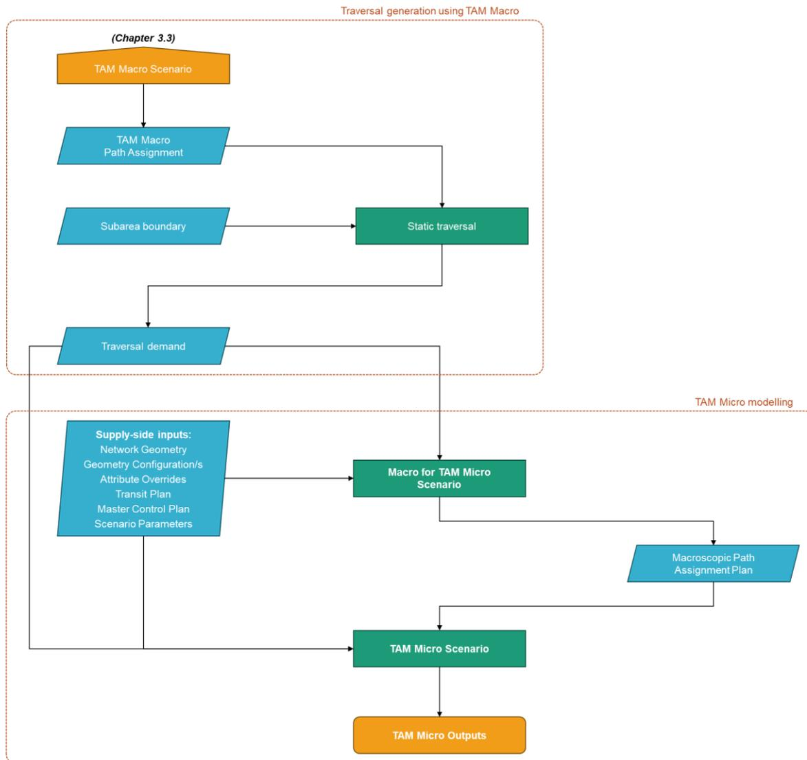
Figure 3.5-1 Overview of the inputs, processes and outputs for a TAM Micro scenario
