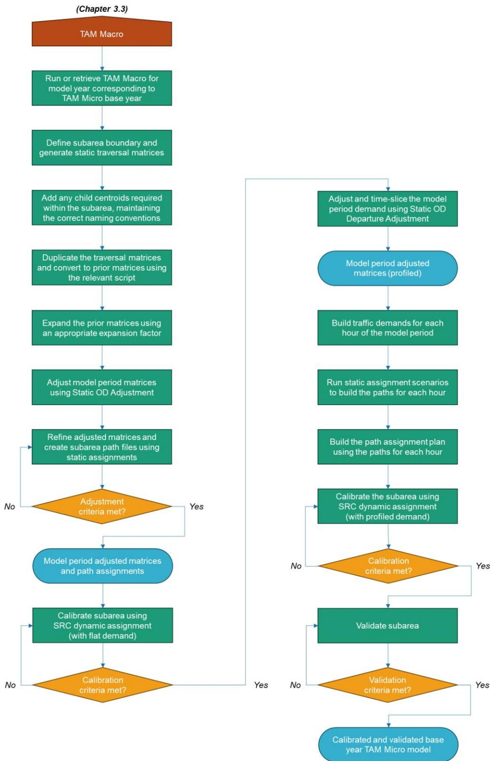
Figure 3.5-7 Base model calibration and validation process for a TAM Micro model
