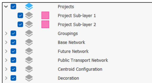
Figure 3.2-3 Example of the creation of project sub-layers in the TAM layer structure
