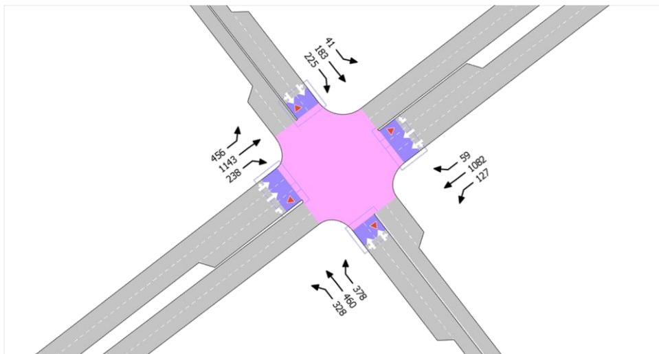
Figure 2.3-1 Example of turning movement data extracted for an intersection
