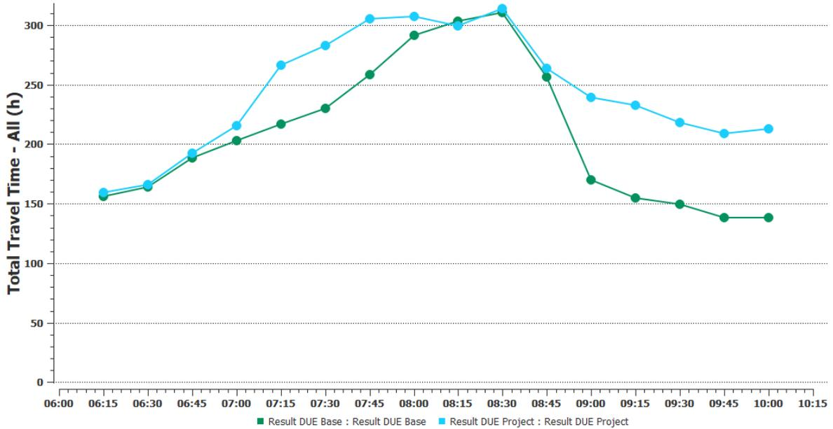
Figure 3.4.4-2 Comparison of total travel time from two different experiment results using Time Series Viewer
