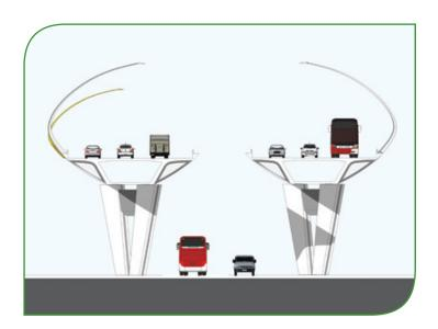
Figure 7: Artist's impression of Superway design and typical cross sections
