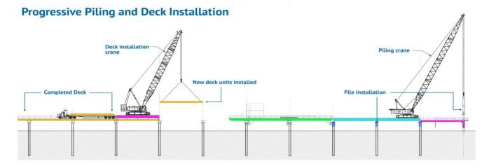
Commencing at the Victor Harbor landing and moving towards Granite Island, a progressive system of piling and deck installation will be used. A leading "front" crane will drive and install the piles, with a second crane following and laying precast concrete decking onto the newly installed piles. A total of 82 steel piles and 85 precast concrete decks will be installed.
