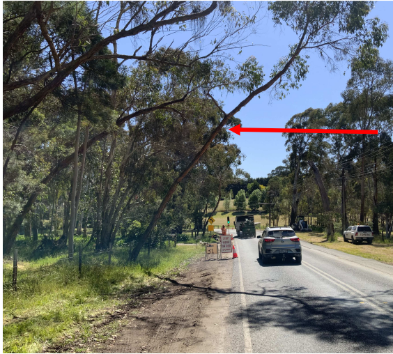
Example of a tree protruding into vegetation clearance envelope that must be removed
