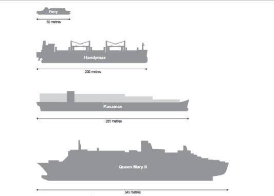
Figure 47: Comparative indication of vessel sizes (EIS Figure 21-9)
