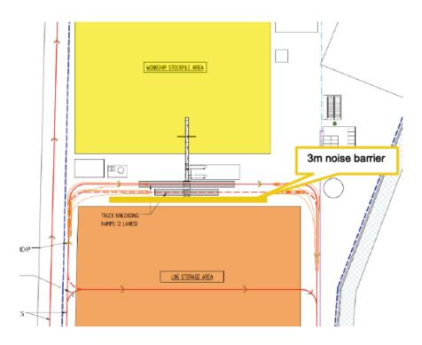
Figure 29: Recommended (Resonate) additional noise barrier (EIS Appendix N Figure 6)
