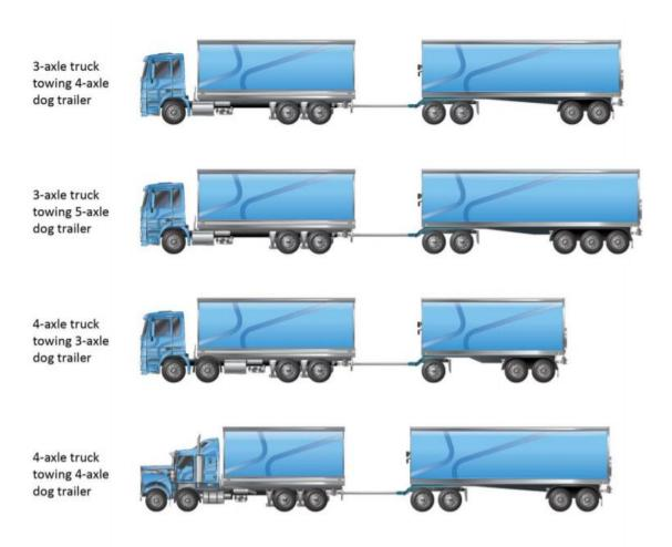
Figure 52: Proposed truck and dog combinations (National Heavy Vehicle Regulator - National PBS Truck and dog trailer notice Information Sheet – May 2016)
