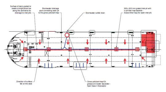
Figure 14: Wharf/barge surface water management system (EIS Figure 4-6)
