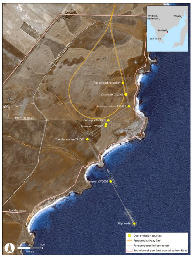
Figure 10-4 Modelled Locations of Air Emission Sources at the Proposed Port Site
