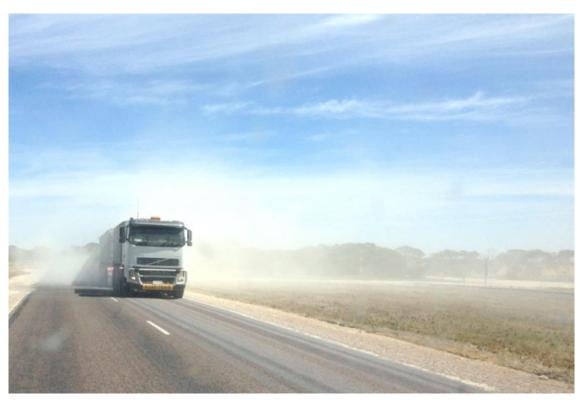
Plate 10-3 Truck-Generated Dust on Sealed Road
