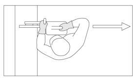
Do not stand in line with the cutting wheel.
