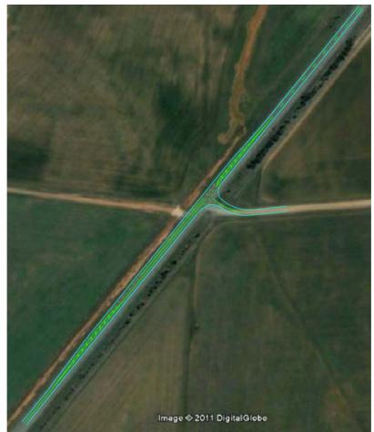
Figure 9: Lipson Cove Road proposed junction treatment
