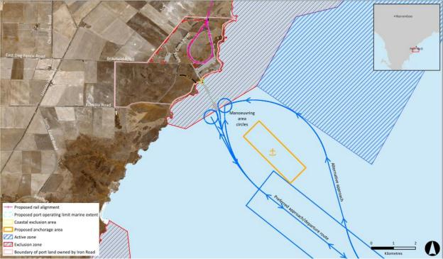
Figure 3-3 Proposed Port layout depicting preferred vessel approach vectors, anchorage areas and turning basins
