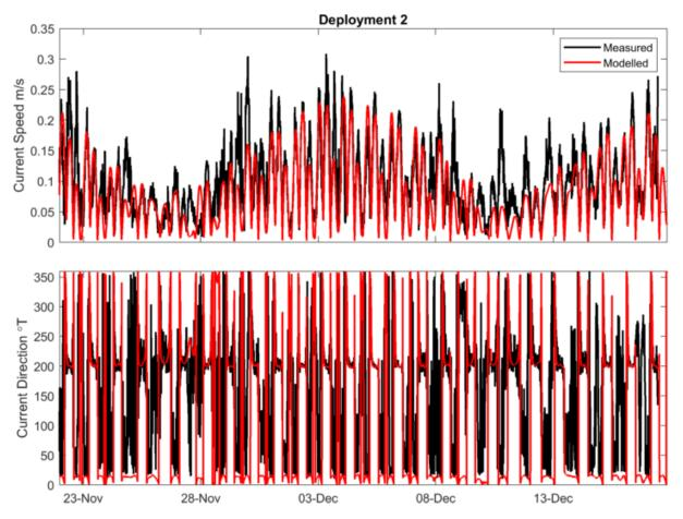
Figure 3.10: Comparison between current speed and direction measured by the ADCP during deployment 2 (Grant *et al.*, 2011) and the coupled hydrodynamic and wave Delft3D model.
