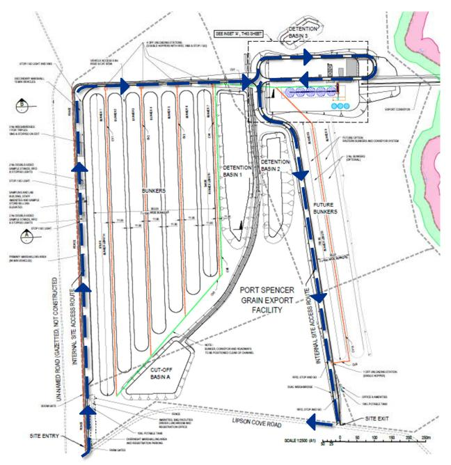
Figure 29: Port Spencer site access arrangement from Lipson Cove Road with indicative internal site circulation (blue dashed line)
