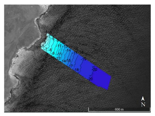
Figure 3.1: Nearshore bathymetric data provided by the client.
