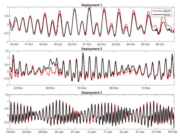
Figure 3.8: Comparison between sea level measured by the ADCP over 5 deployments (Grant *et al.*, 2011) and the coupled hydrodynamic and wave Delft3D model.
