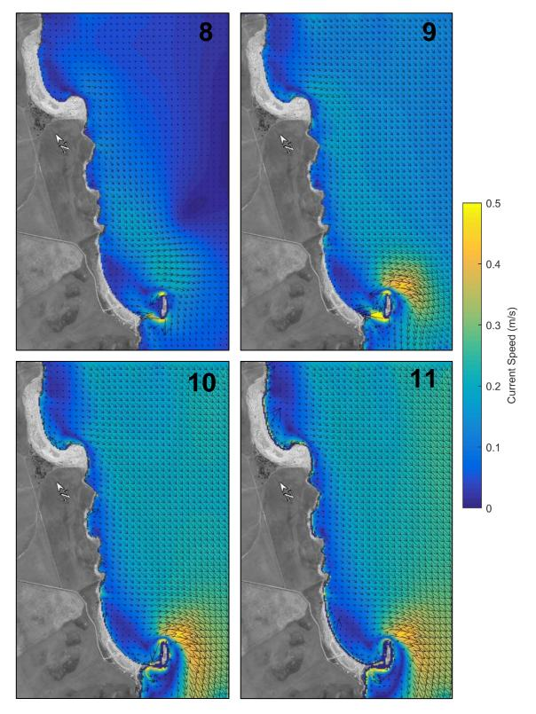
Figure 4.7: Currents speeds during hours 8 to 11 of the tidal cycle.
