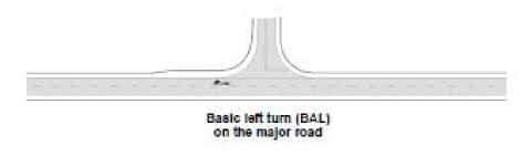
Figure 31: Example of a basic left turn (BAL) treatment from major road (Source: Austroads)
