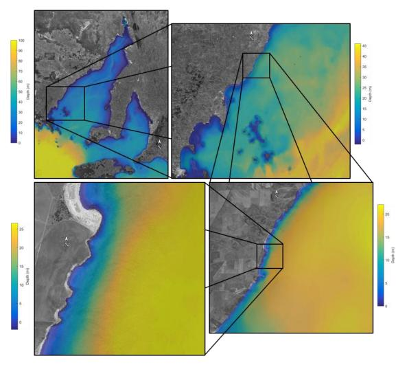
Figure 3.3: Nested bathymetry grids used for the Swan wave model.
