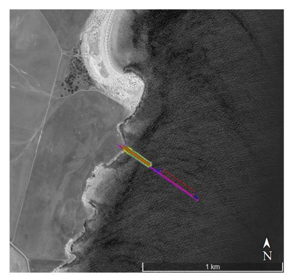
Figure 1.2: The layout of the proposed development with causeway (brown/yellow), the wharf (magenta) and the outline of the berthed ship (red).
