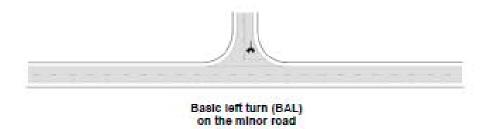
Figure 32: Example of a basic left turn (BAL) treatment from minor road (Source: Austroads)
