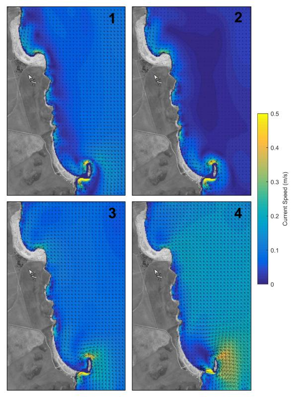
Figure 4.5: Currents speeds during hours 1 to 4 of the tidal cycle
