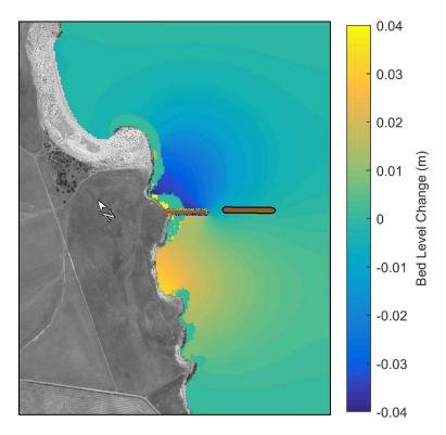
Figure 4.12: Difference in annual sediment accumulation and erosion patterns between baseline and post development scenarios for a grain size of 0.13 mm. Positive values indicate increased accumulation and negative values indicate increased erosion due to the presence of the development.
