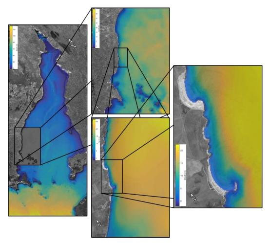
Figure 3.7: Nested bathymetry grids used for the Delft3D coupled hydrodynamic and wave model wave model.
