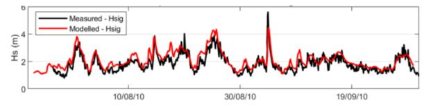
Figure 3.4: Comparison between significant wave height measured by the ADCP (Doubell *et al.*, 2015) and the SWAN wave model.
