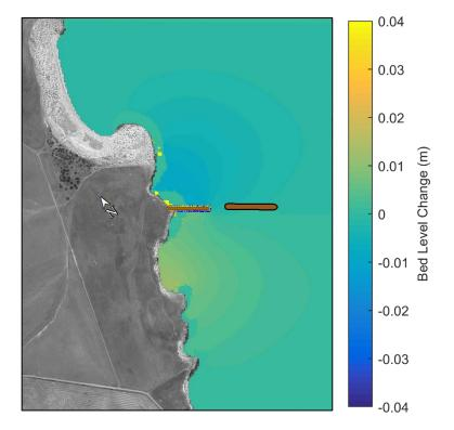
Figure 4.11: Difference in annual sediment accumulation and erosion patterns between baseline and post development scenarios for a grain size of 0.3 mm. Positive values indicate increased accumulation and negative values indicate increased erosion due to the presence of the development.
