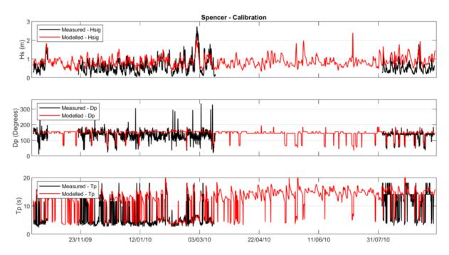
Figure 3.5: Comparison between waves measured by the ADCP (Grant et al., 2011) and the SWAN wave model.
