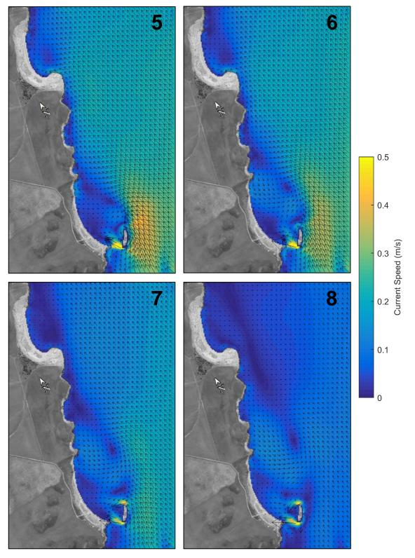
Figure 4.6: Currents speeds during hours 5 to 8 of the tidal cycle
