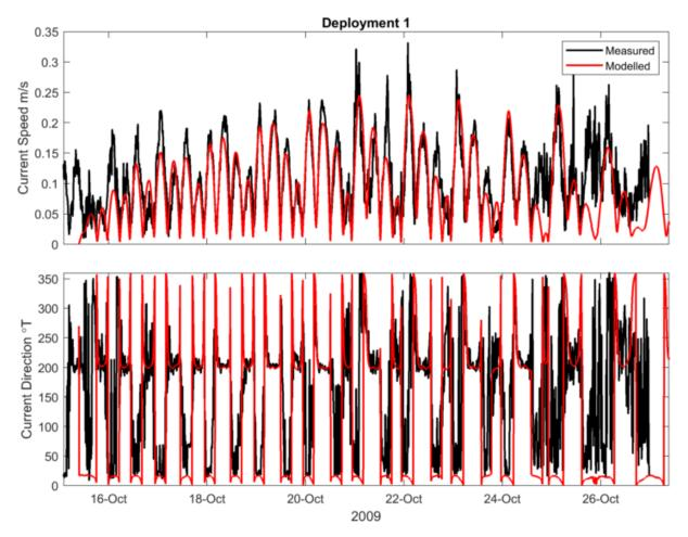
Figure 3.9: Comparison between current speed and direction measured by the ADCP during deployment 1 (Grant *et al.*, 2011) and the coupled hydrodynamic and wave Delft3D model.
