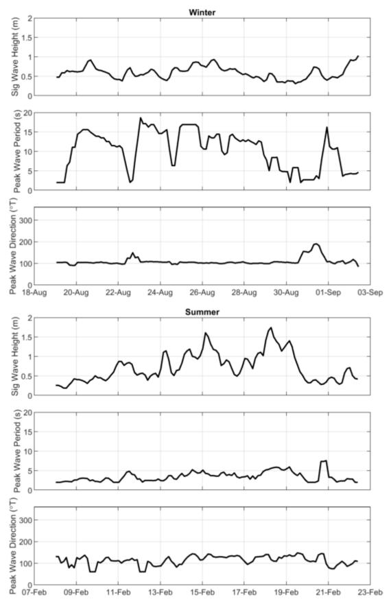
Figure 3.12: Winter (top) and Summer wave height, period and direction boundary conditions for sediment transport modelling.
