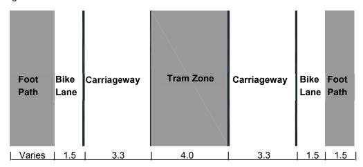
Figure 11 Required Cross section for Option 2 on the Eastern approach on The Parade prior to the intersection
