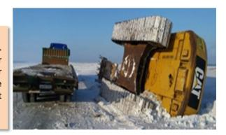
What Could Have Happened? Without effective controls such as the restricted work area or effective cab design & protection, a fatality or serious injury could have resulted.
