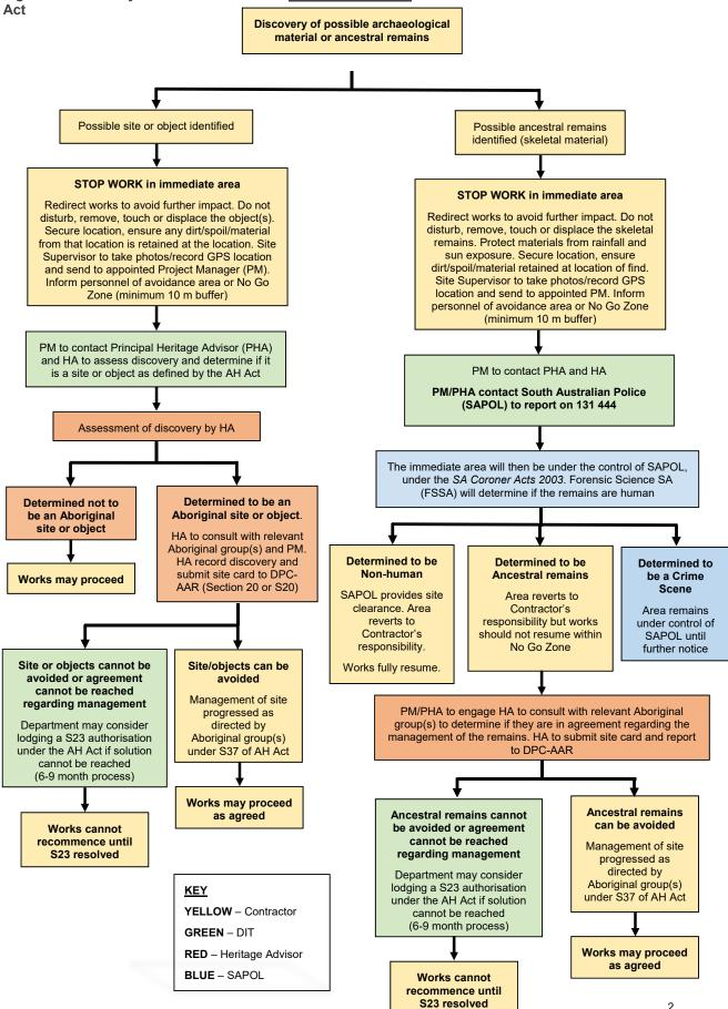
Figure 2 - Discovery Procedure Flow Chart with Section 23 Authorisation under the AH Act
