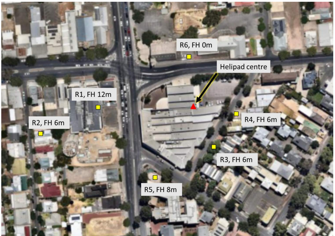
Figure 9: Discrete receptors (yellow square symbols) and nominated flagpole heights (FH). FH expressed as metres above ground.
