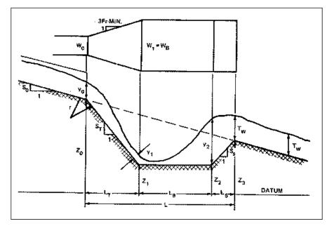
Figure 6: Flow Definition sketch for Free Jump Energy Dissipation Basin (USDOT, 2006)
