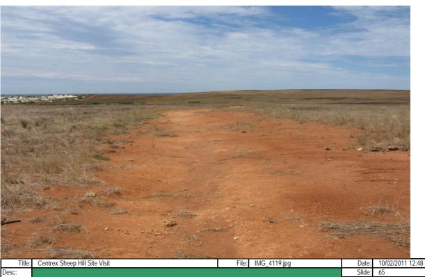
Site 10: Facing south-east. Same location as Slide 64. Looking downstream onto Centrex property. Measured cross-section of drainage course: Top width 3 m, depth about 15 cm. Very little loose soil. Consolidated silty, sandy-clayey. Low flat area and Roger's Beach in left background.
