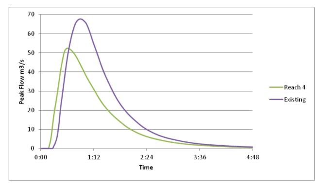
Figure 7: Comparison of 100 Year ARI Peak Flow Event for the 1 hr Storm Duration for the Existing and Proposed Offsite Conditions
