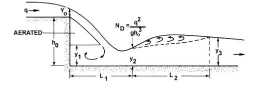
Figure 4: Flow Geometry of a Straight Drop Spillway (USDOT, 2006)
