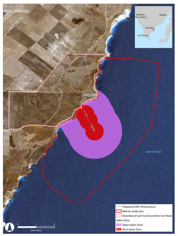
Figure 14-9 Observation and Shut-Down Zones
