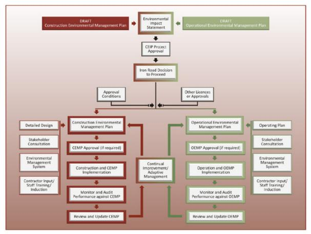
The process for approval and review of the construction and operational EMPs is shown in Figure 1-2.
