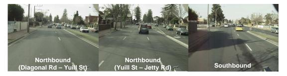
■ **Section 3**: Diagonal Road to Oaklands Road – this section consists of 2 traffic lanes in both the northbound and southbound directions within a typical road width of 19m.
