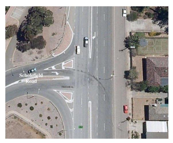
Figure 6-12: Existing Layout of Brighton Road / Scholefield Road / Ocean Boulevard Junction
