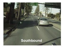
■ Section 2: Jetty Road (Glenelg) to Diagonal Road – this section consists of 2 traffic lanes between Diagonal Road and Yuill Street and 3 traffic lanes between Yuill Street and Jetty Road in the northbound direction, and 2 traffic lanes in the southbound direction within a typical road width of 20m.
