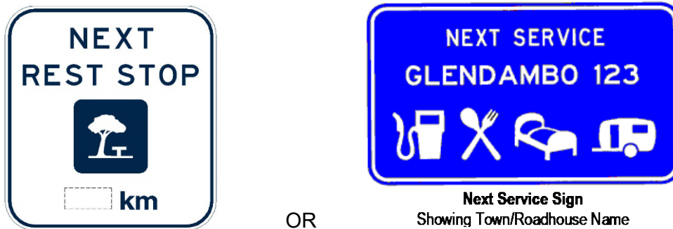
Figure 3.2: Examples of “Next Rest Stop” and “Next Service” signs
