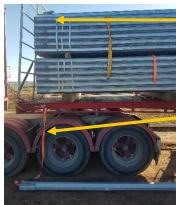
The securing straps were cut by the telehandler operator, releasing the stored energy potential.
