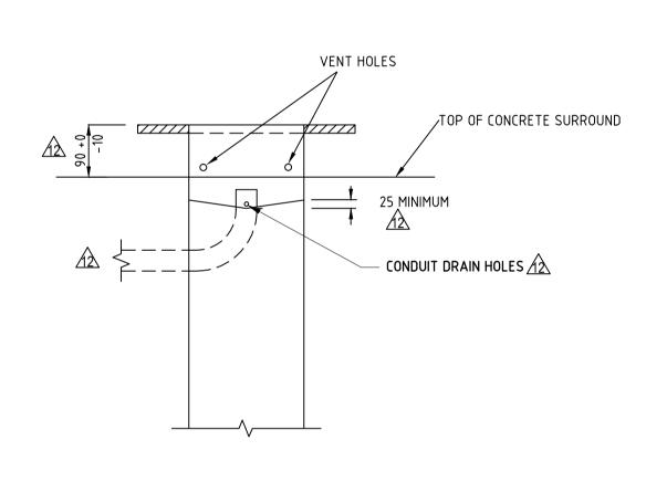
DETAIL A FOOTING UNIT INSTALLATION-TYPICAL REFER TO NOTES THIS SHEET
