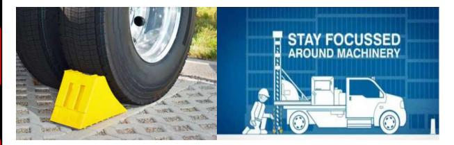
A number of Australian workers have been seriously injured or killed because vehicles haven't been safely immobilised while work is being done on or around them. Duty holders must ensure trucks, trailers, and mobile plant are safely immobilised when they exit these vehicles or work around them.
