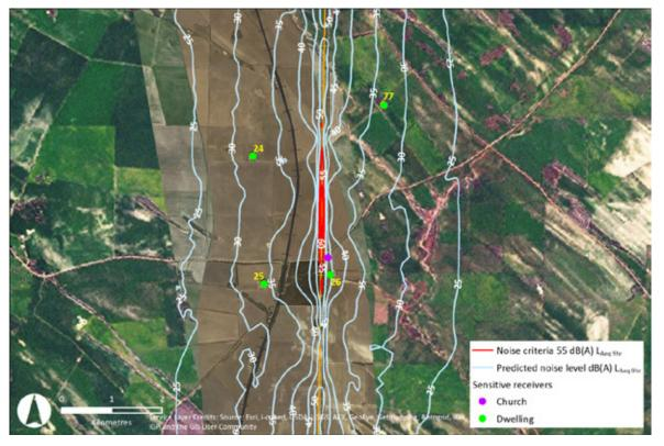
Figure 12-6 Example Enlargement of the Predicted Noise Contours, Night  $L_{Aeq 9hr}$  for the Operation of the Railway
