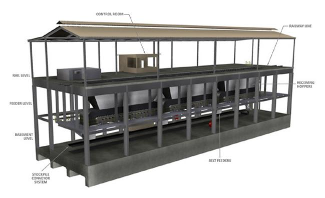
NOTE: THIS FACILITY WILL BE ENCLOSED WITH CLADDING AND FITTED WITH DUST CONTROL UNITS TO CAPTURE RESIDUAL DUST
