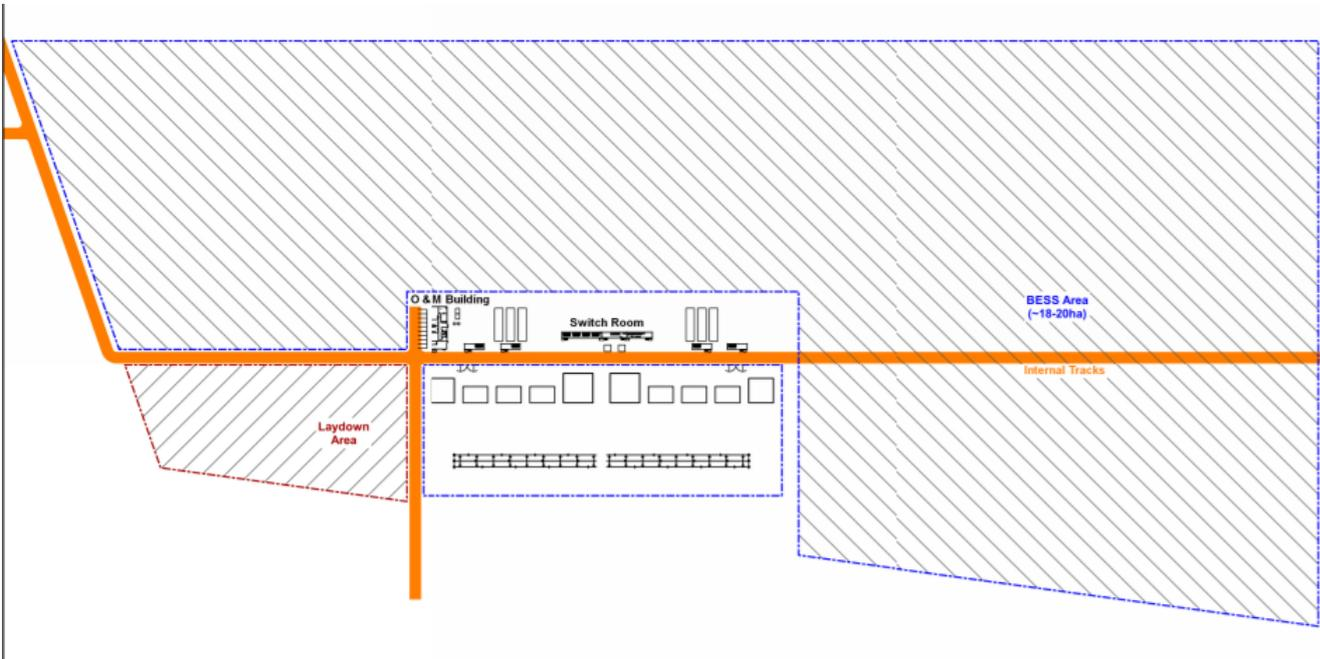
Figure 11: Indicative BESS, project substation and site office area layout
