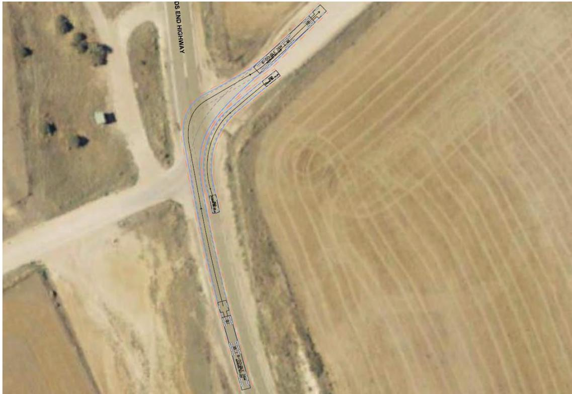
Figure 4.5: 26 Metre B-Double Turn Path - Left Turn from Powerline Road
