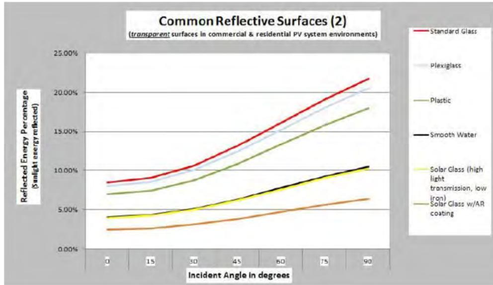
Figure 3: Reflected Energy in % of sunlight (Detail)
