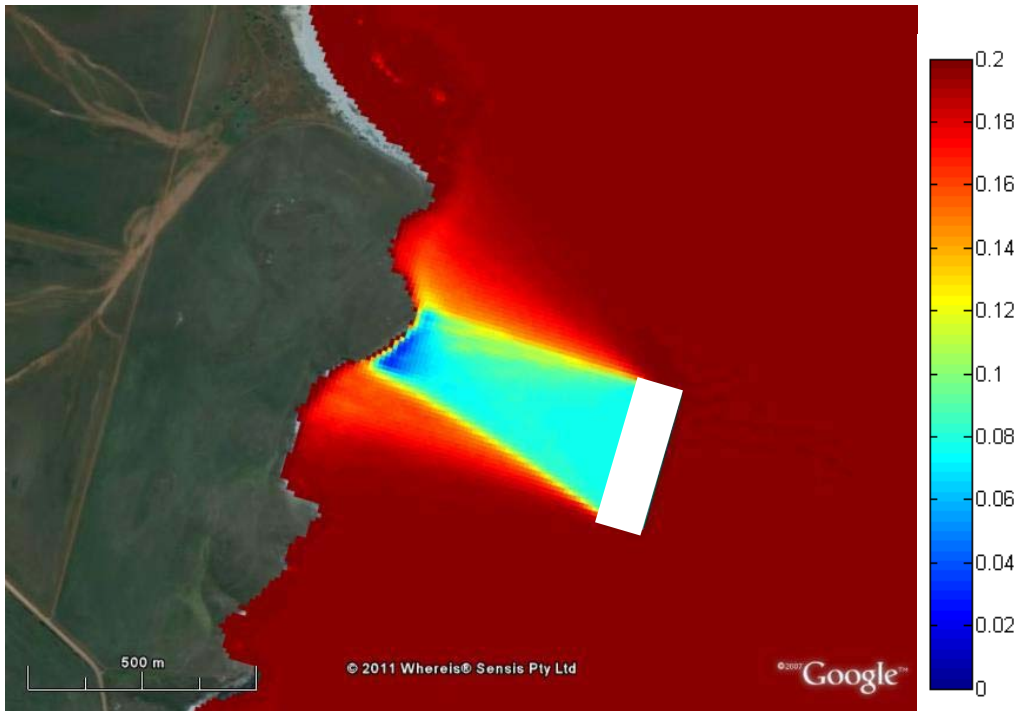
Figure 4.3. Predicted difference in wave height (m) due to moored vessel for winter conditions. White rectangle represents vessel.
