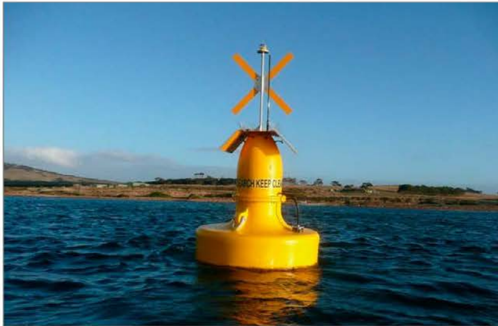
Figure 2-4 Water quality monitoring buoy (BMT)
