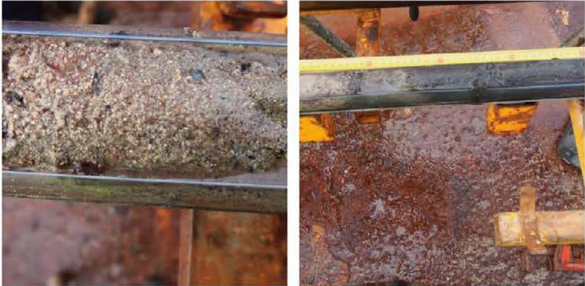
Figure 5-1 Sediment cores from COOE (2017) sampling. Left – prevailing silty sand material, showing relatively coarse grain size. Right – sandy silt material with high organics content from SB7.2
