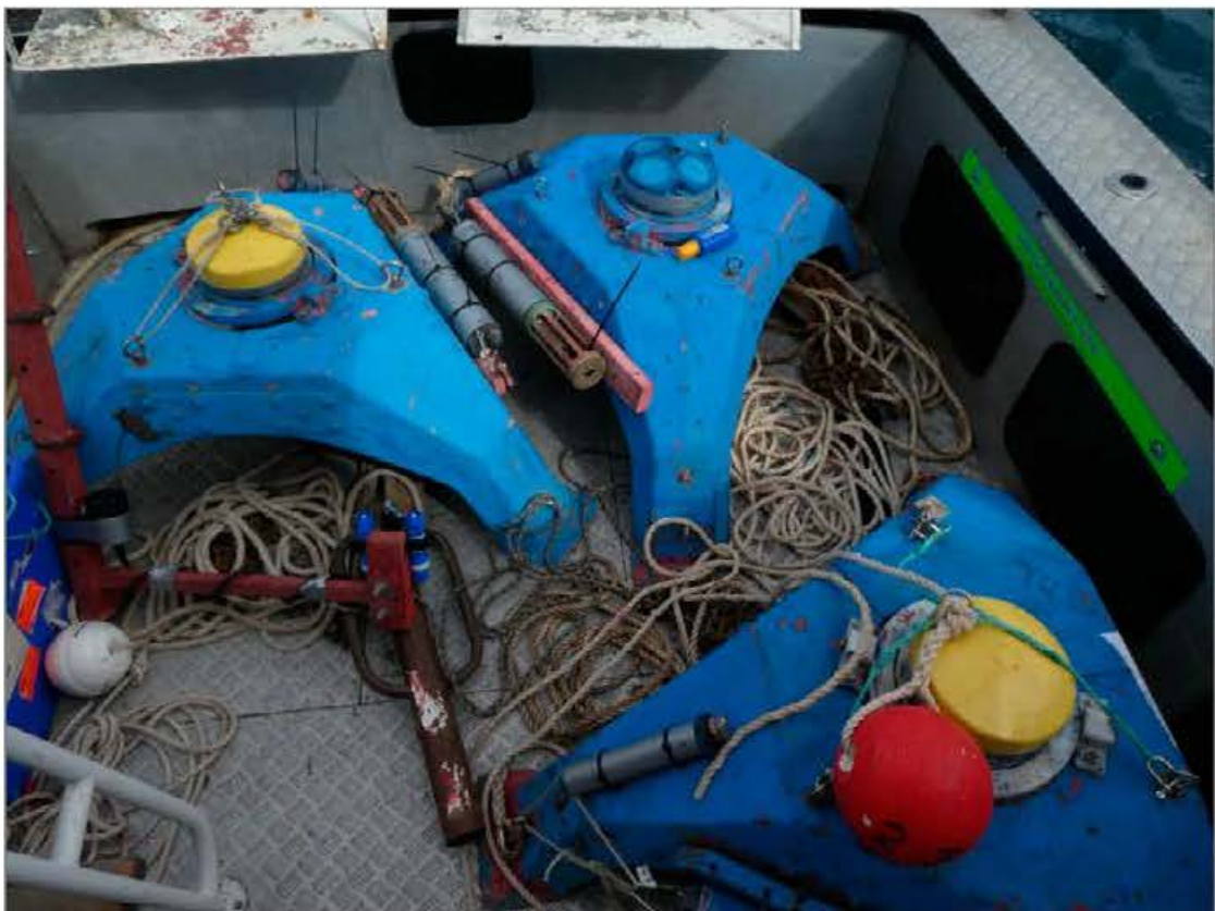
Figure 2-5 Instrument deployment using bottom-mounted frames
