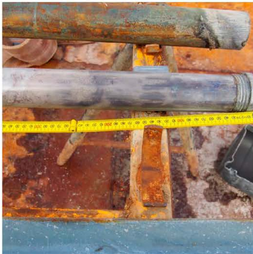
Photo 2. Sediment core in PVC tube recovered from metal drill bit
