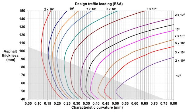
Figure RD-PV-D2 7-2 Allowable Traffic Loadings of Asphalt Overlay for Projects with WMAPT of 25-30°C and without Existing Asphalt
