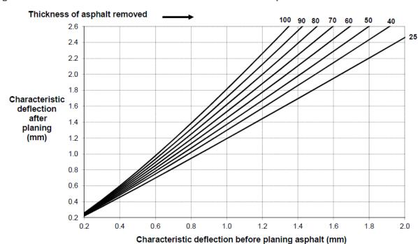
Figure RD-PV-D2 7-3 Increase in deflection due to removal of asphalt
