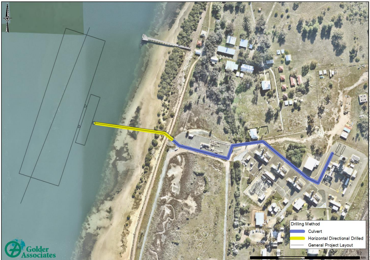
Figure 10: Pipeline alignment showing installation method
