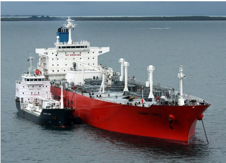
Figure 1: An example of Origin's floating storage and gas transfer operation at Moreton Bay, off Brisbane Port.
