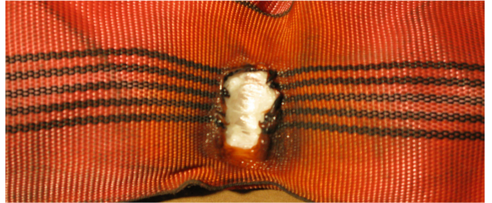
Heat and friction damage
