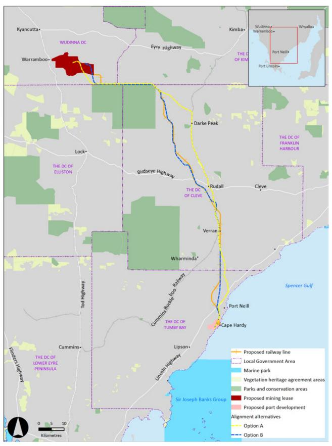
Figure 3-2 Railway Line Alignment Alternatives
