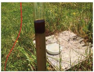
Photograph 13: Showing a grab sample from the disused septic with LNAPL sitting above liquid waste
