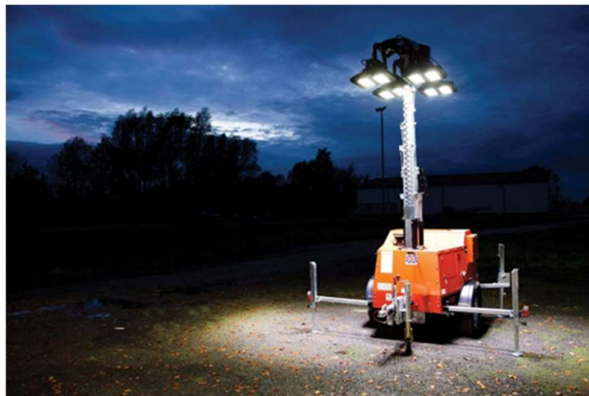
An example of a light tower used for night works.
